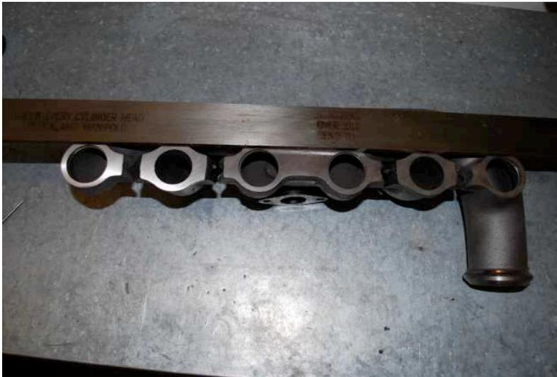
The standard exhaust manifold carries all the weight of the muffler and tail pipe. Over time this weight and the heat generated in the exhaust manifold causes the cast iron in the manifold to sag unless gland rings are installed.
