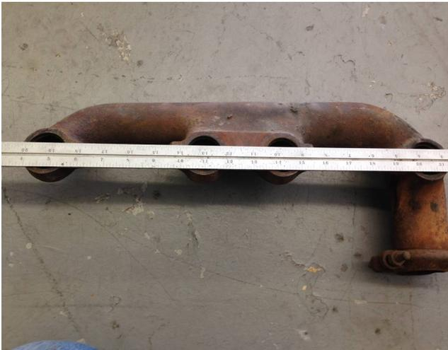
This photo shows how to lay a straight edge across the exhaust ports. You must carefully set the edge starting at the #1 port then working across to #2 then #3. You want to set it exactly at the bottom of each port, starting with #1. Then you see how #4 looks. It will generally show a gap due to distortion of the manifold.
