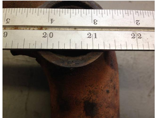
Close up of #4 Port, this manifold is no good, should be scrapped. Gland rings will not fit and it will leak at #4 Port. Anything over  $1/32''$  misalignment will keep you from installing the gland rings.
